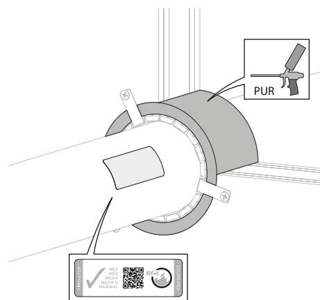
5. Slide the collar into the opening of the wall, in the middle of the wall thickness.
