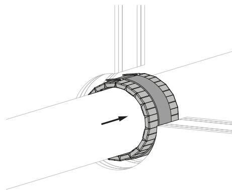
4. Slide the collar into the opening of the wall, in the middle of the wall thickness.
