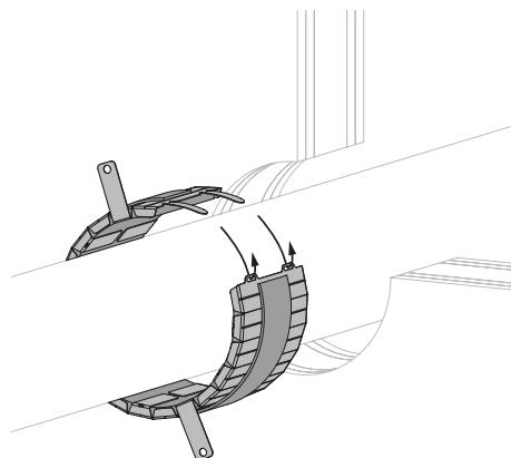
3. Fold the metal plates with pre-drilled holes for 270°.
