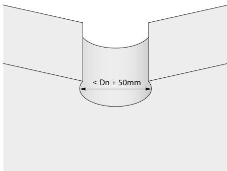
1. Provide an installation opening of  $\leq \text{Ød} + 50 \text{ mm}$ .
