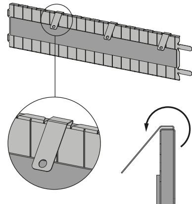
2. Fold the metal plates with pre-drilled holes for  $300^\circ$ .
