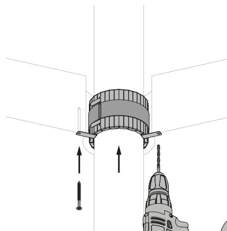
4. Slide the collar into the opening until it reaches the height of the ceiling.
