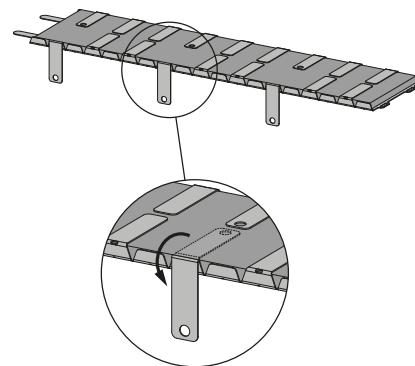
2. Fold the metal plates with pre-drilled holes for  $270^\circ$ .
