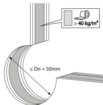
2. Provide an installation opening of  $\leq \text{Ød} + 50 \text{ mm}$ .
